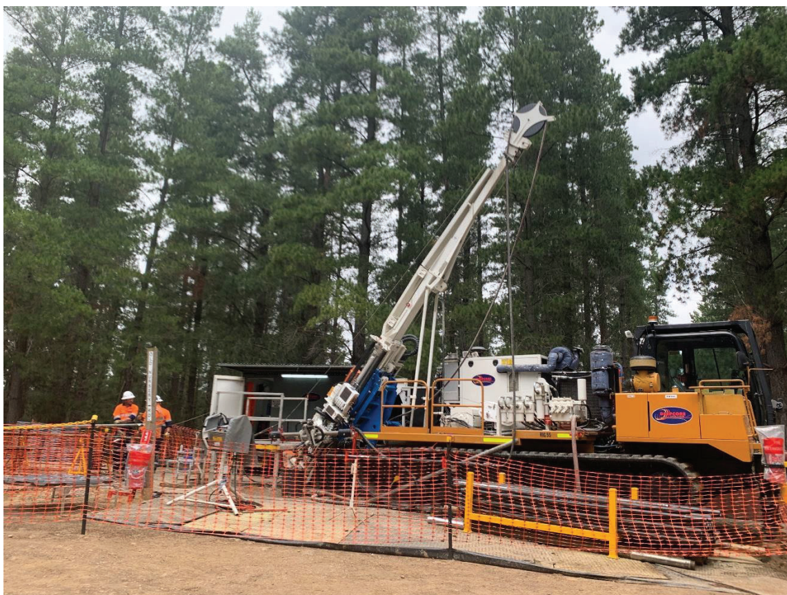
Figure 2: Diamond Drill Rig at the Castlemaine Gold Project
