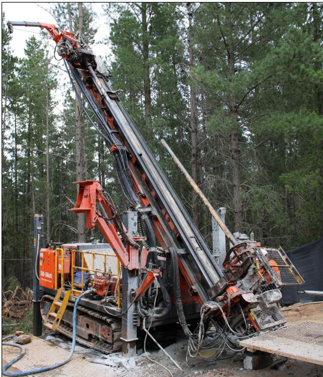
Figure 3: Diamond drill rig in operation at the Lightning Prospect
