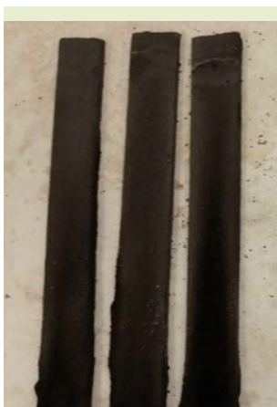
First Graphene FireStop™ 450 micron 2 coats
