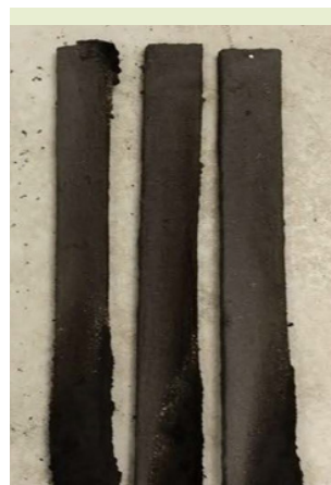
First Graphene FireStop™ 700 micron 3 coats
