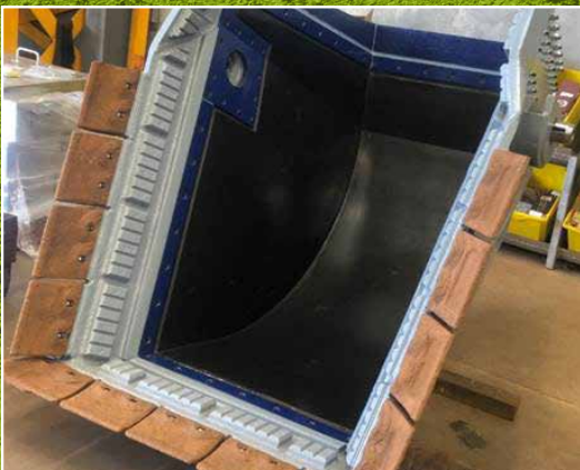
Reclaimer bucket liner enhanced with ArmourGRAPH™
