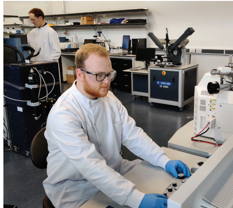
Adam Smalley (Research Technician) in the foreground carrying out scanning electron microscopy (SEM) and Dr Tom Raine (Senior Development Chemist) in the background using the thermogravimetric analyser (TGA) in the Analytical Lab at the GEIC.
