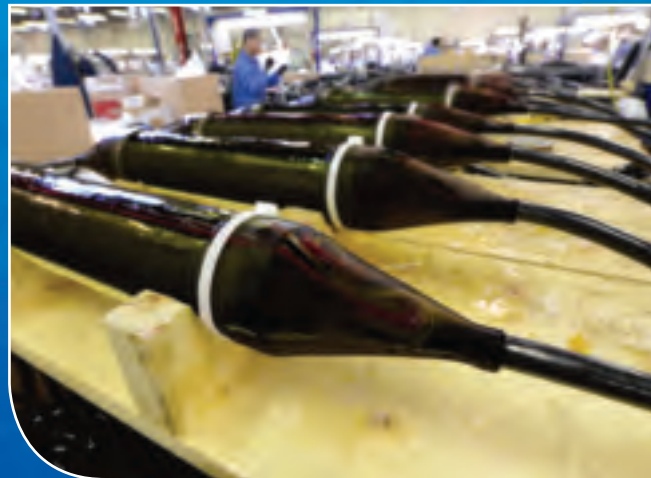
Seismic sensors are attached to the cable and permanently sealed in protective cases creating sensor pods at specified intervals along the PRM cable sections.
