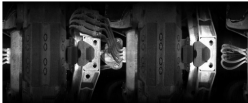
Ultra-High Definition Undercarriage Image at 46 MPH
