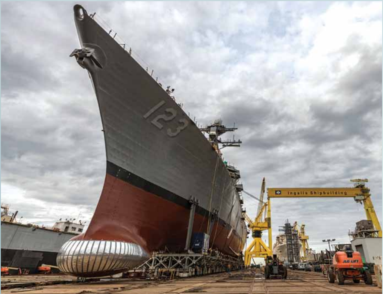
Lenah H. Sutcliffe Higbee (DDG 123) is the 34th Arleigh Burke -class destroyer constructed at Ingalls Shipbuilding.
