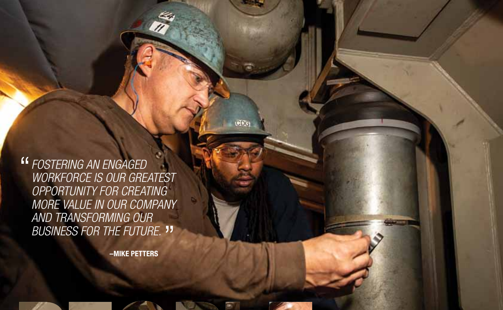
Ingalls Shipbuilding employees (L-R) Randall Bailey and Carlos Grant take depth readings to ensure tolerances are correct.
