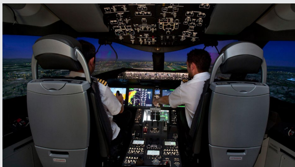
L-3's 787 full flight simulator is the first in the world to be qualified with a fully functional avionics capability, including an electronic flight bag and heads-up display.
