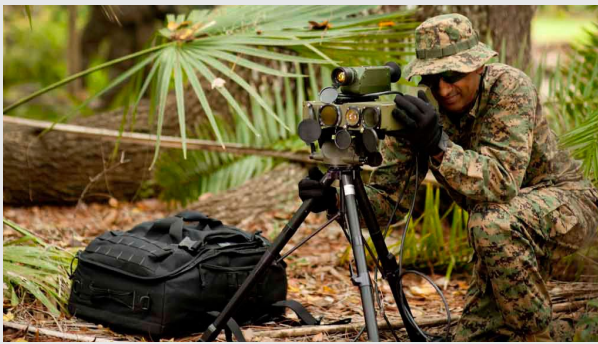
L-3's new Scarab system is a modular laser designator equipped with rangefinding and an IR thermal imager, providing accurate target designation, both day and night, and in nearly all battlefield conditions.
