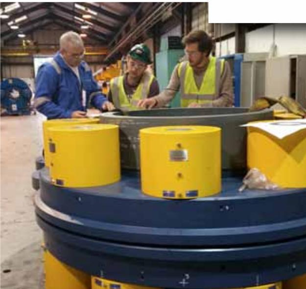
**POS-GRIP HGSS™ Subsea Wellhead components are assembled for testing**
