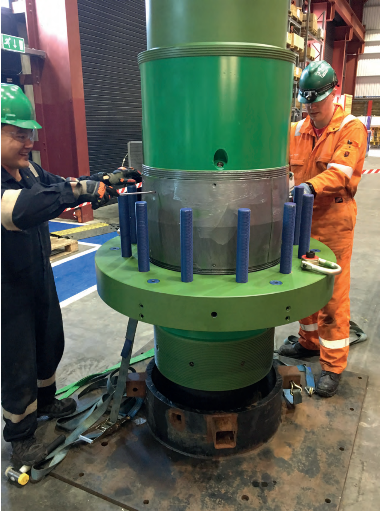
POS-GRIP "HG" production wellhead is assembled ready for testing ahead of drilling and producing a new North Sea well
