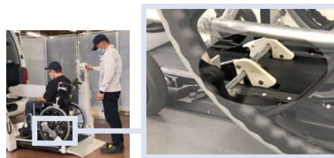
The one-touch wheelchair fastening device being developed by Toyota. The white hooks at the center of the righthand photo latch onto the wheelchair's anchor bar to secure it in place, with the entire process taking just two seconds once the switch is pressed.
