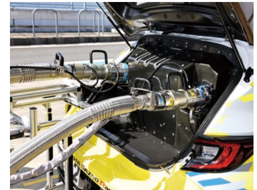
Refueling with liquid hydrogen
