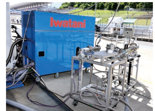
Mobile liquid hydrogen station developed by Iwatani Corporation and Toyota
