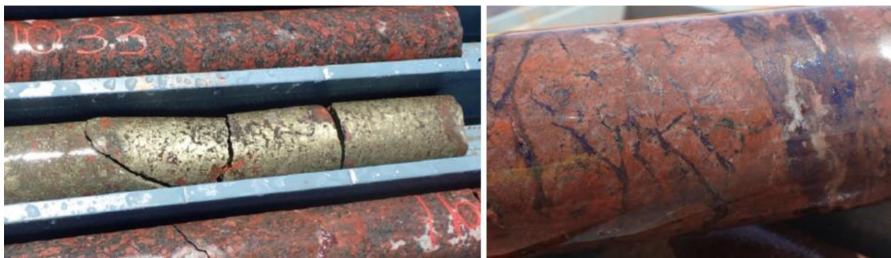
Figure 4: Pervasive chalcopyrite + pyrite mineralisation in altered, hematite-rich granite (left hand photograph) and bornite + chalcopyrite stringers in hematite-rich, altered granite (right hand photograph).
