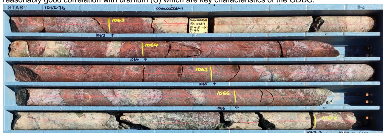
Figure 4: Granite (hematised) with cross-cutting, quartz + sericite altered intrusives. Chalcopyrite mineralisation at 1,063.68m assayed 5.07% Cu and 0.78 g/t Au over 0.32m.
