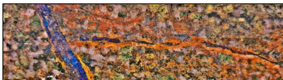
Figure 9: HWDD08 939m Bornite vein with siderite and orange feldspar rim.
