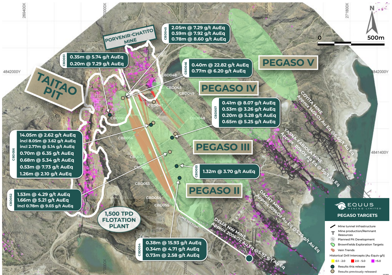
Figure 6 – Plan view showing summary Pegaso II Target drill results and interpreted intersected vein trends and B-B' long section (presented in Figure 7)
