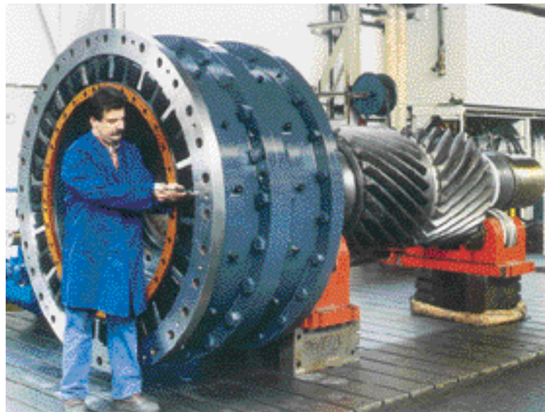
A 25-tonne Renold Hi-Tec coupling being installed at Mannesmann's steel works in Germany
