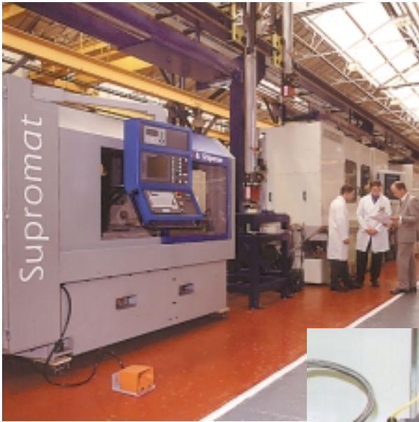
Renold's group-wide expertise at work. New automated production line including Holroyd and Jones & Shipman machine tools, using Manifold indexers for work placement.
