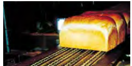
Lubrication free chains are used in hygiene critical food production industry.
