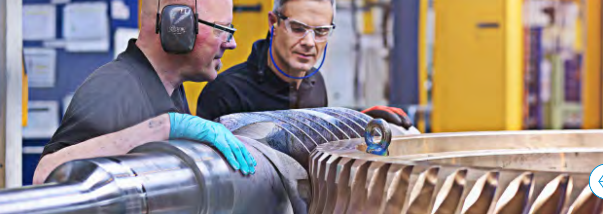
Pictured: At our Gears facility in the UK, pairing of large worm gear sets used in coal crushers.
