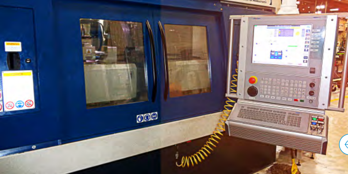
Pictured: The addition of the Sinico machine in our US Chain facility allows quick and precise production of pins with many customised features such as cut-ins, off-sets, extensions, shoulders and threading.
