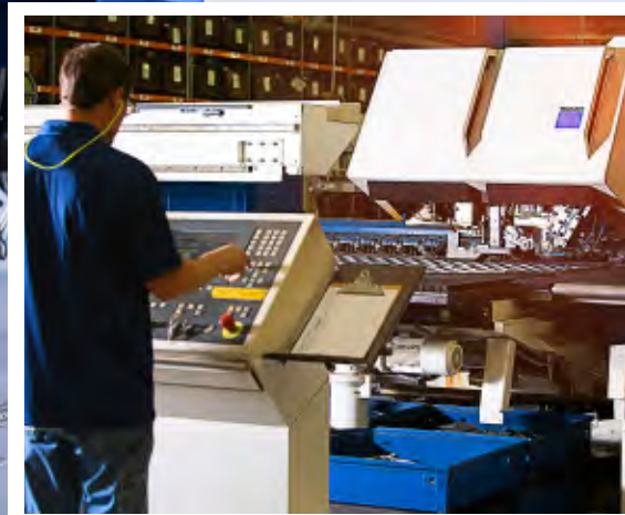
Pictured: At our US Chain facility, the Trumpf laser cutter is able to cut sidebars with speed and form precision attachment chain with a variety of features such as bends, chamfered edges and grooves.
