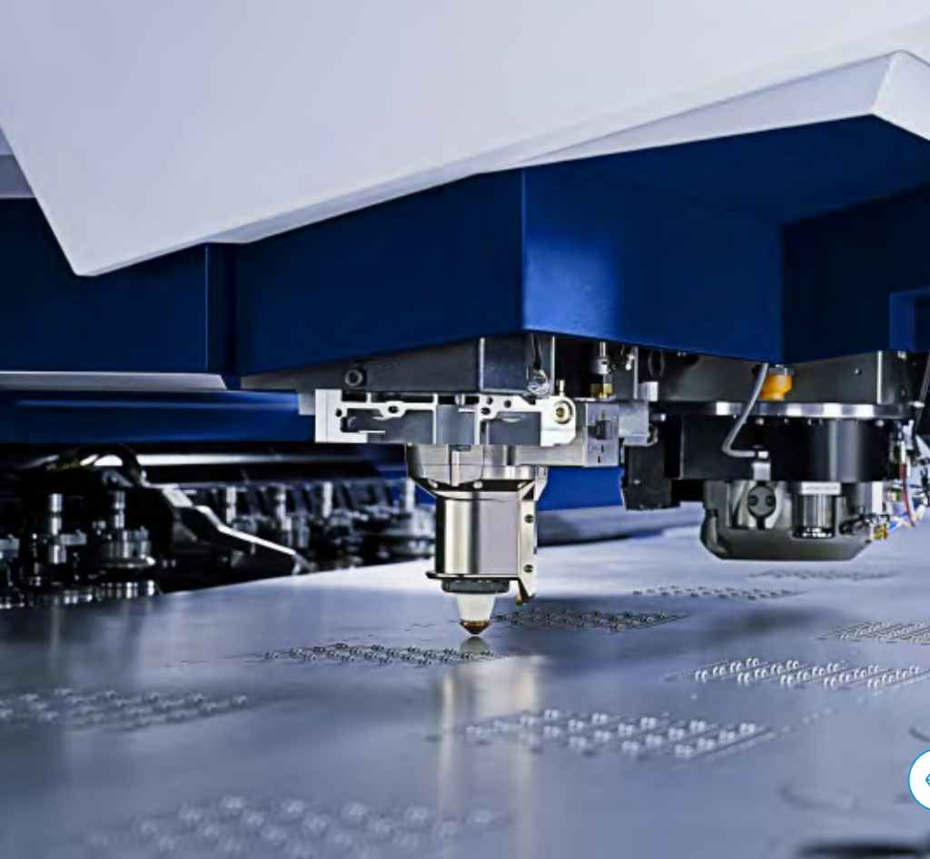
Pictured: At our US Chain facility, the Trumpf laser cutter is able to cut sidebars with speed and form precision attachment chain with a variety of features such as bends, chamfered edges and grooves.
