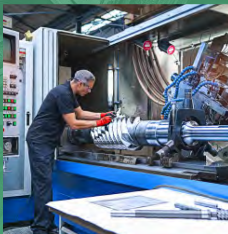
Pictured: Worm thread grinding of large worm gears for use in coal pulverisers in coal fired power stations.
