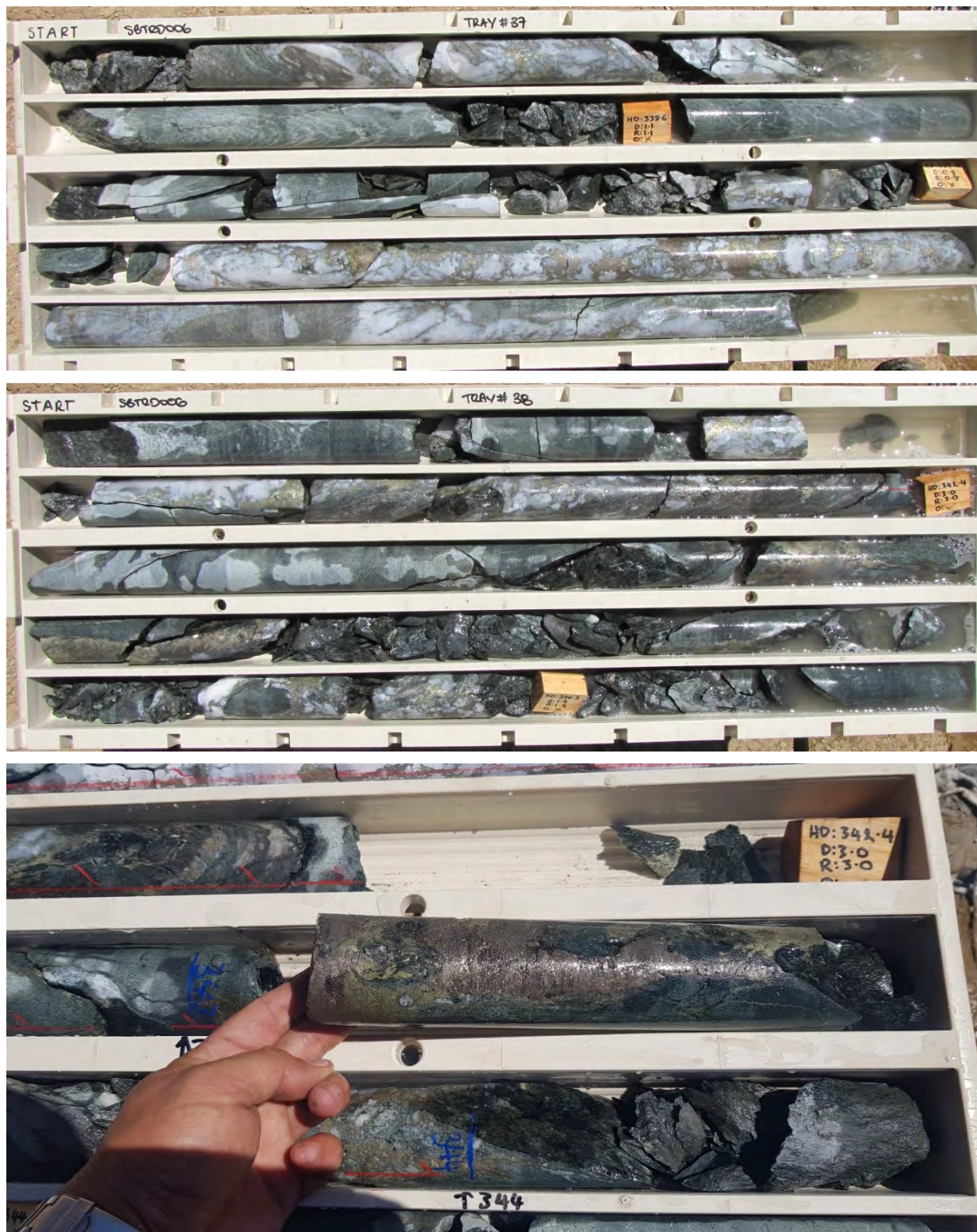
Figure 19. Bottletree SBTRD006 core: Top and middle photographs showing Trays 37 and 38 containing drill core from down hole depths 337m – 341.5m (approx.) and 341m – 344.5m (approx.) respectively, showing strong chalcopyrite and pyrite mineralisation. Bottom photograph shows close-up view of drill core from 343m (approx.).
