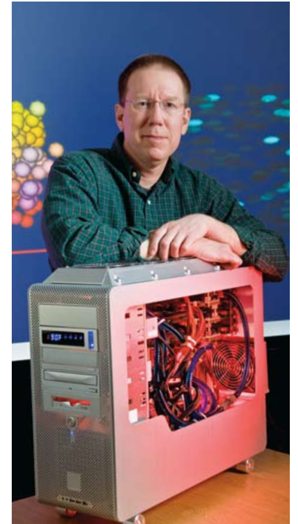
Dr. Jack Collins displays a computer system he developed for the National Cancer Institute that uses a series of graphic processors for tackling drug design problems, such as screening hundreds of thousands of candidate drug molecules. Each candidate drug now can be screened in minutes instead of the hour it used to take using a more expensive computer cluster.
