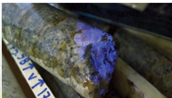
Quartz veining with coarse scheelite in core from the 2015 drilling program
