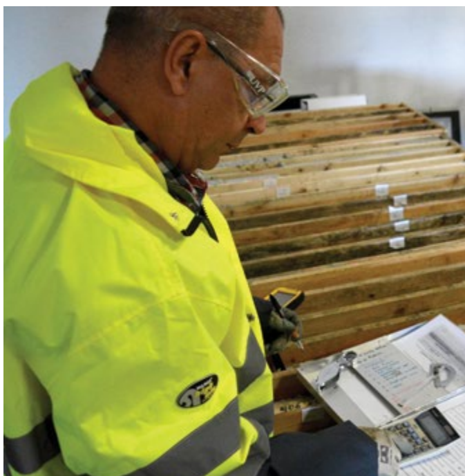
Logging of core from the 2015 drilling program
