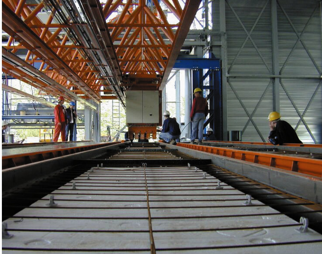
Above: In 2001, Dycore commissioned a new highly automated factory at Lelystad in the Netherlands to manufacture its newly-developed insulated floor elements. These are highly insulated prestressed units cast in self-compacting concrete, which exceed the strict Dutch regulations for thermal insulation in new houses. Pictured is the first test-pouring with self-compacting concrete.
