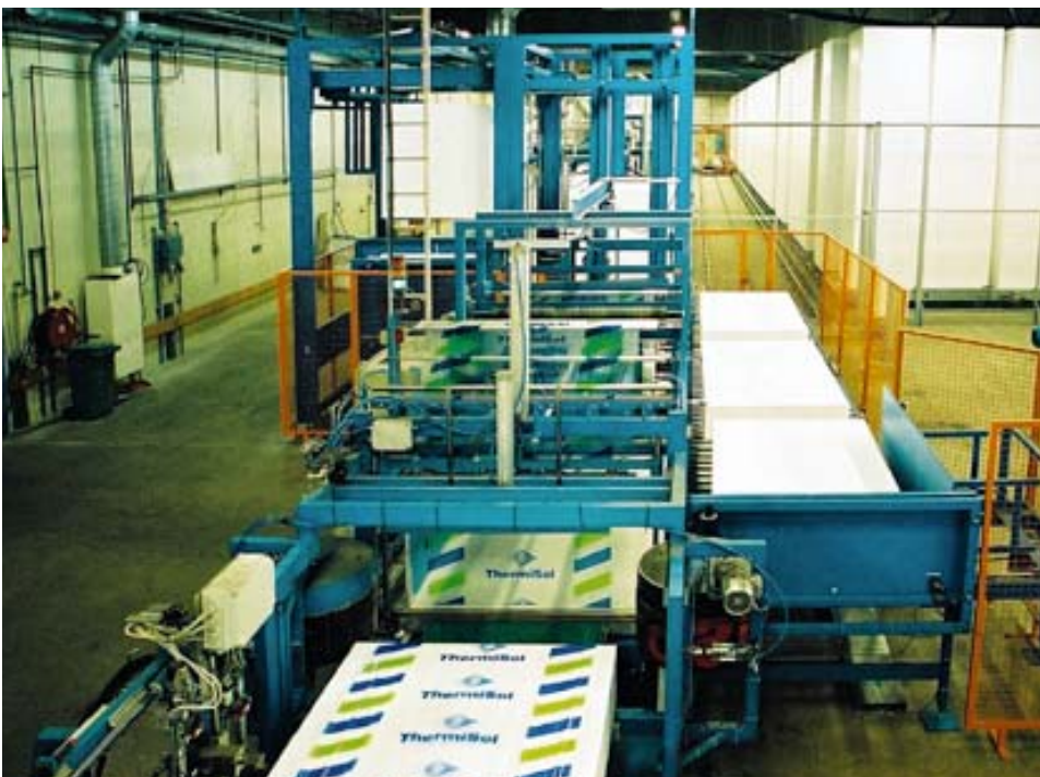
The new state-of-the-art, fully automated expanded polystyrene insulation plant recently installed in ThermiSol Sweden's Norrtälje facility.
