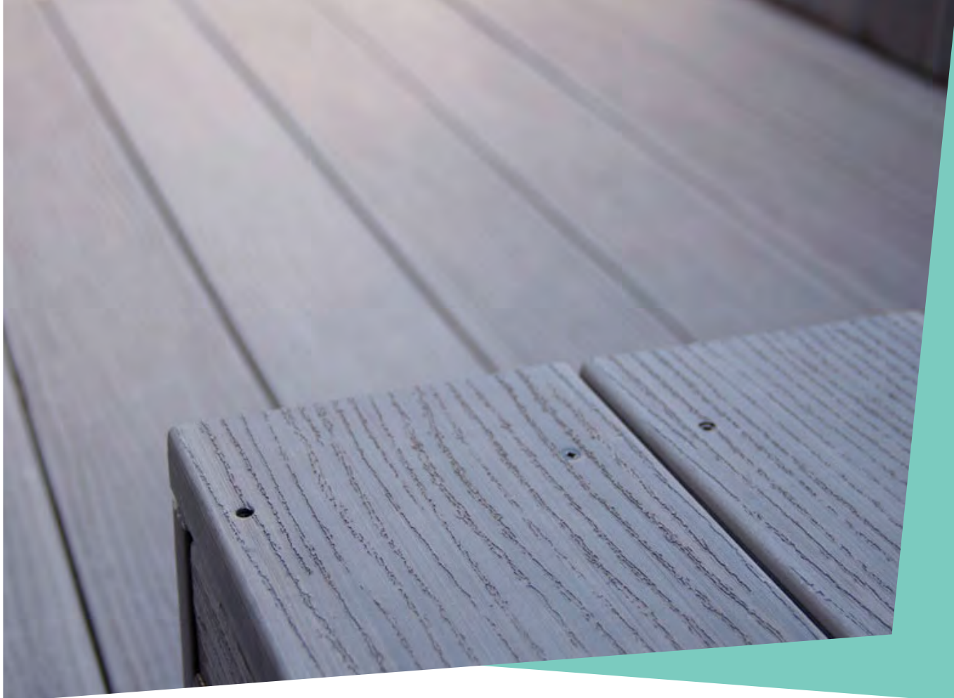
Decks in PVC with phenolic waste particles
