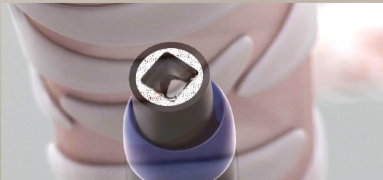
Creo's concept Fibre Optic Probe based Raman Spectroscopy aims to use infra-red to instantly diagnose unhealthy tissue structures.
