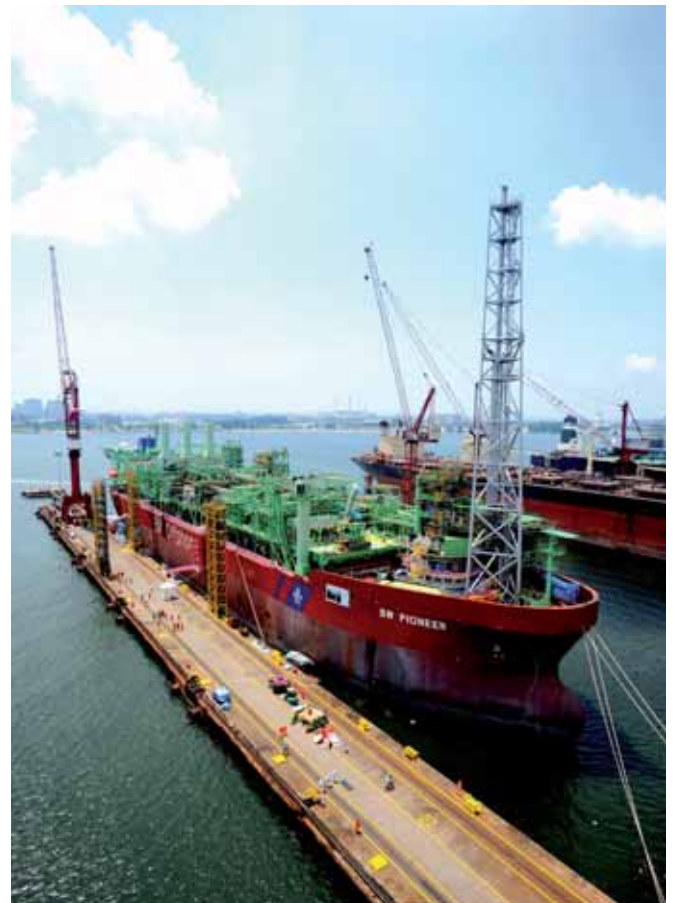
BW Pioneer will be the first FPSO to be deployed in the Gulf of Mexico and turret moored at the deepest waters ever for an FPSO.
