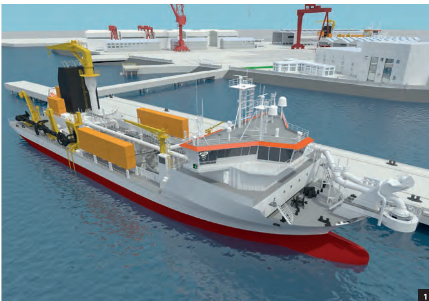
1. Keppel Singmarine is building the world's first EU Stage V dredger in compliance with stricter international limits on emissions.
