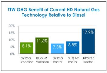
For the CWI ISX12 G, ISL G and ISL G Near Zero engines, the tailpipe  $CO_2$ , methane, and  $N_2O$  emissions were taken from EPA and CARB certification Executive Orders. HPDI 2.0 attributes are based on Westport internal data. GHG benefits are calculated using the EPA specified methods applicable to Phase 1 GHG Regulations.
