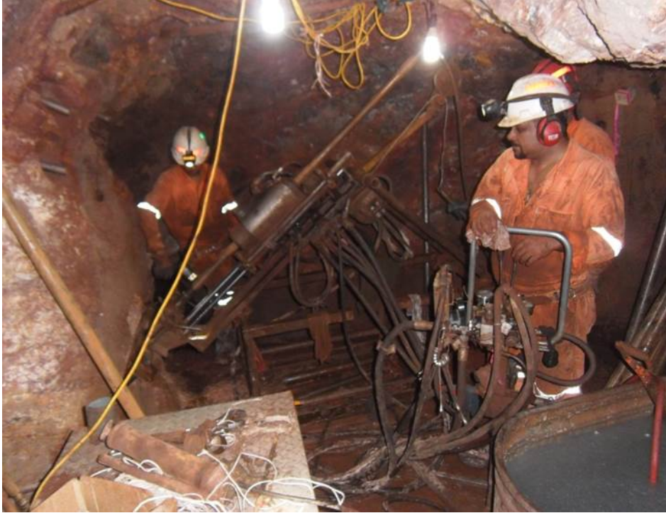
Figure 34. Typical Set-Up of the Termite Drill during the Long Hole Twin Program, 2012-2013
