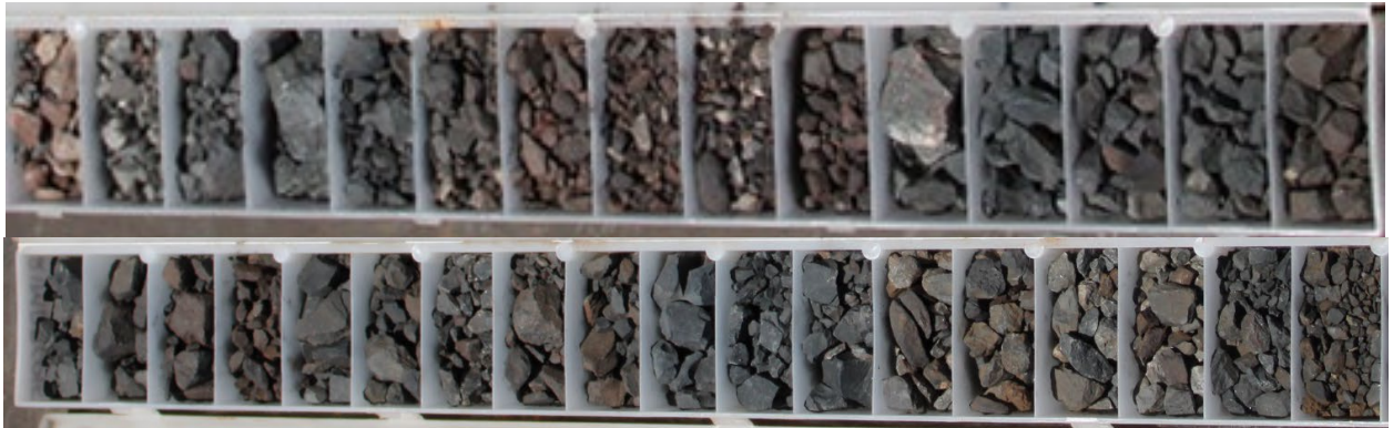
Image 10 / RC drill chips: 21MDRC015 65-76m (11m @ 2.27% Cu & 429ppm Co & 78-98m 20m @ 1.99% Cu & 30ppm Co, chalcocite & covellite mineralisation)
