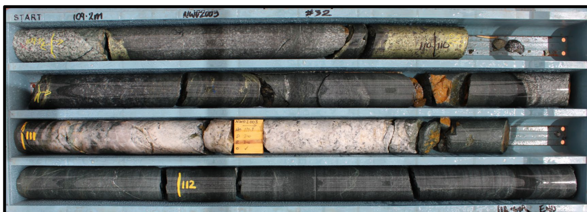
Image 16 | NWD2003: 109.2m to 110.05m; 0.7m @ 6.58% Cu, 2.83 Au g/t and 16.5 g/t Ag
