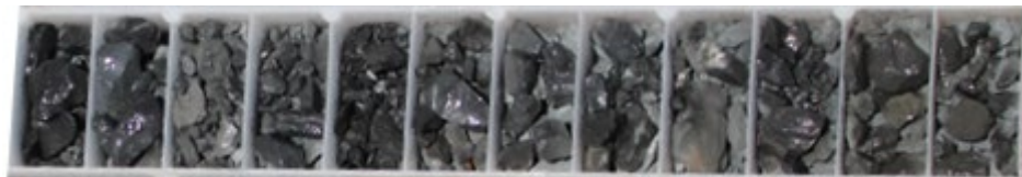
Image 11 / RC drill chips: 21MDRC018 108-117m (9m @ 0.95% Cu & 284ppm Co. pyrite & chalcopyrite mineralisation)
