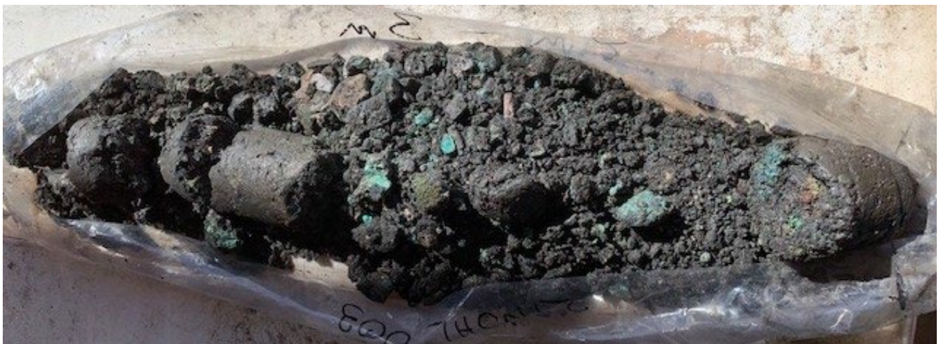
Image 1 | Metallurgical test-work sample from Sonic Rig
