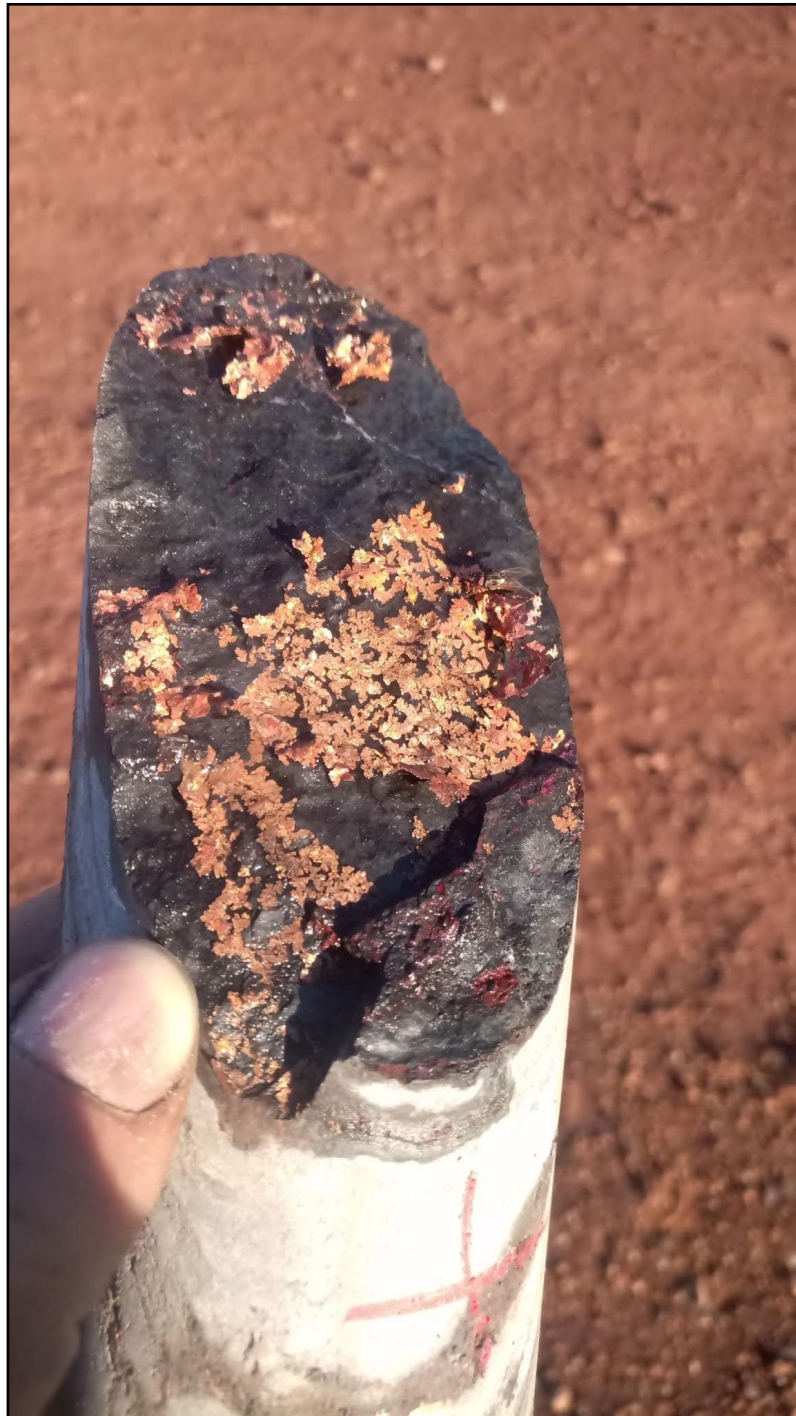
Image 2 | Hole 21NDMT001: 141.4m to 141.5m showing native copper and chalcocite
