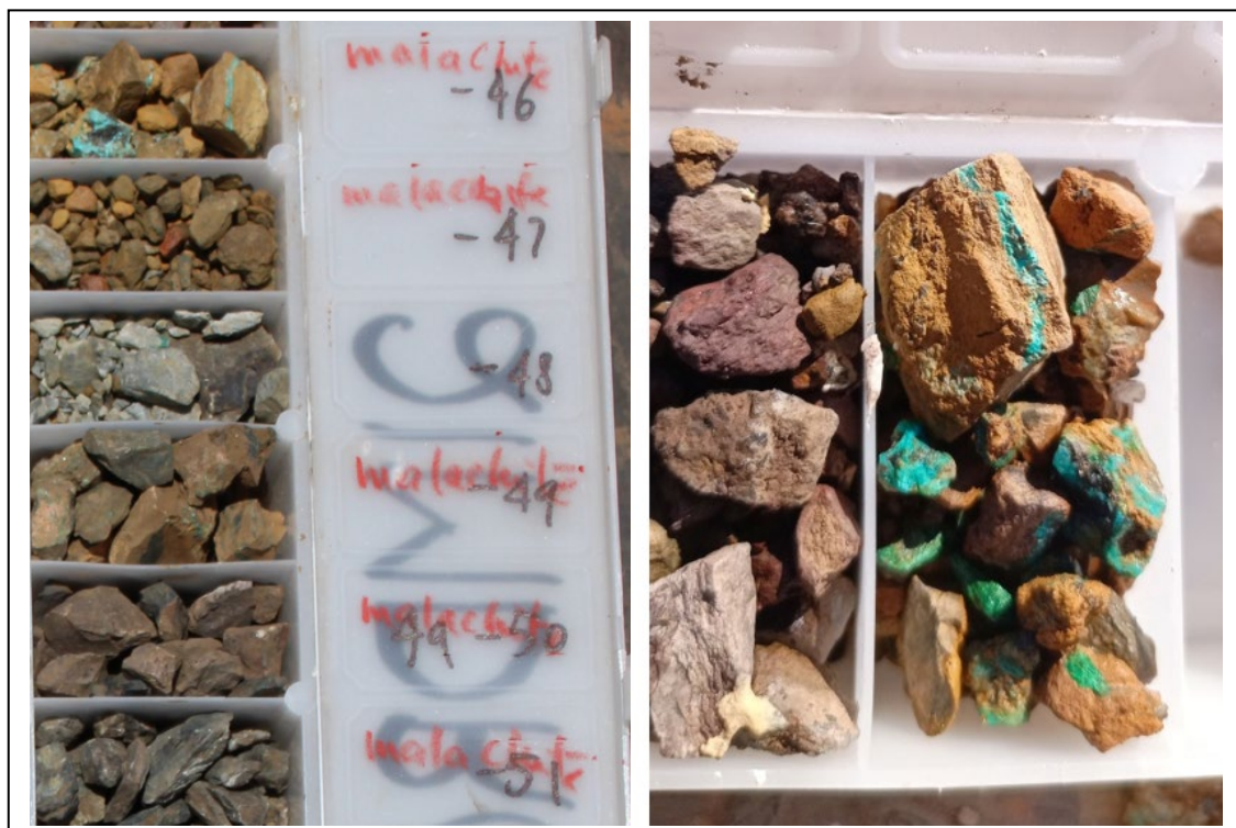
Image 12 | Malachite and Chrysocolla 46-51m 21MDRC016 (9m @ 1.25% Cu & 775 ppm Co from 44m)
