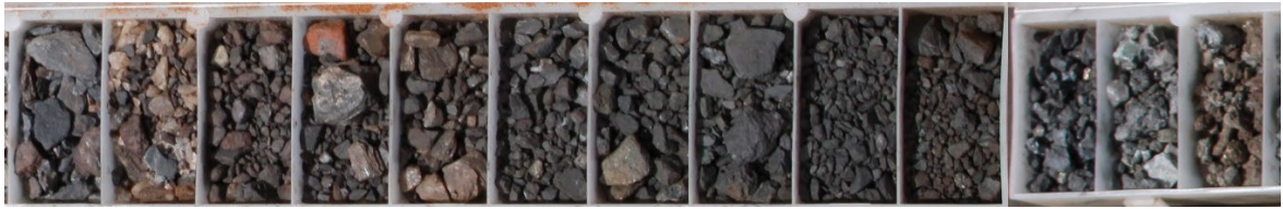
Image 9 / RC drill chips: 21MDRC012, 50-63m (13m @ 0.85% Cu & 429ppm Co, cuprite, chalcocite & covellite mineralisation)
