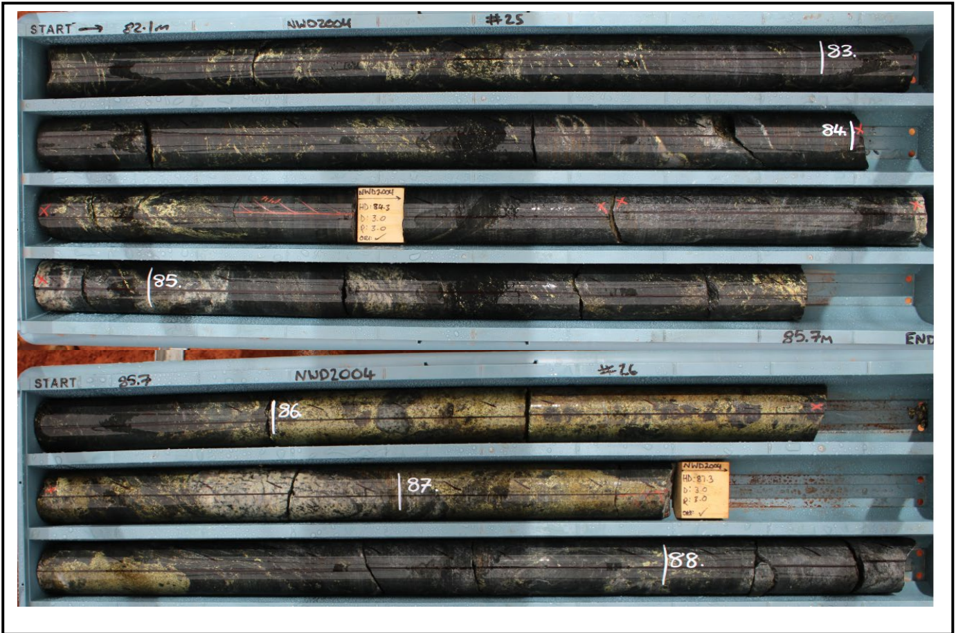
Image 18 | NWD2004: 82.1m to 88.0m; 5.9m @ 3.6% Cu chalcopyrite mineralisation, including 1.0m @ 10.9% Cu from 86.0m
