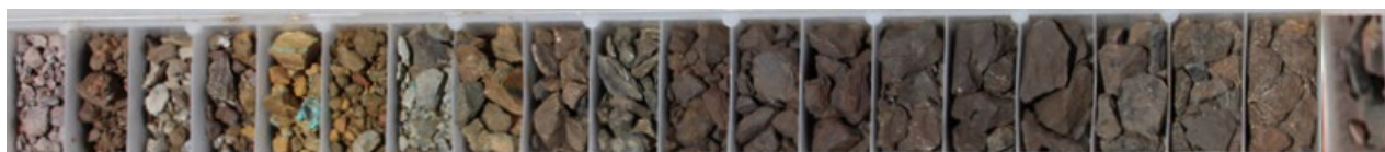
Image 8 / RC drill chips: 21MDRC016 41-61m (20m @ 0.86% Cu & 609ppm Co malachite, cuprite & chalcocite mineralisation)
