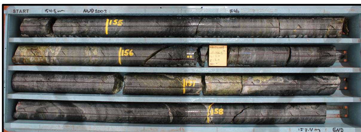
Image 15 | NWD2003: 155.0m to 156.0m; 1.0m @ 5.11% Cu, 0.40 Au g/t and 8.50 g/t Ag. 156.7m to 157.4m; 1.0m @ 11.0% Cu, 0.82 Au g/t and 18.5 g/t Ag
