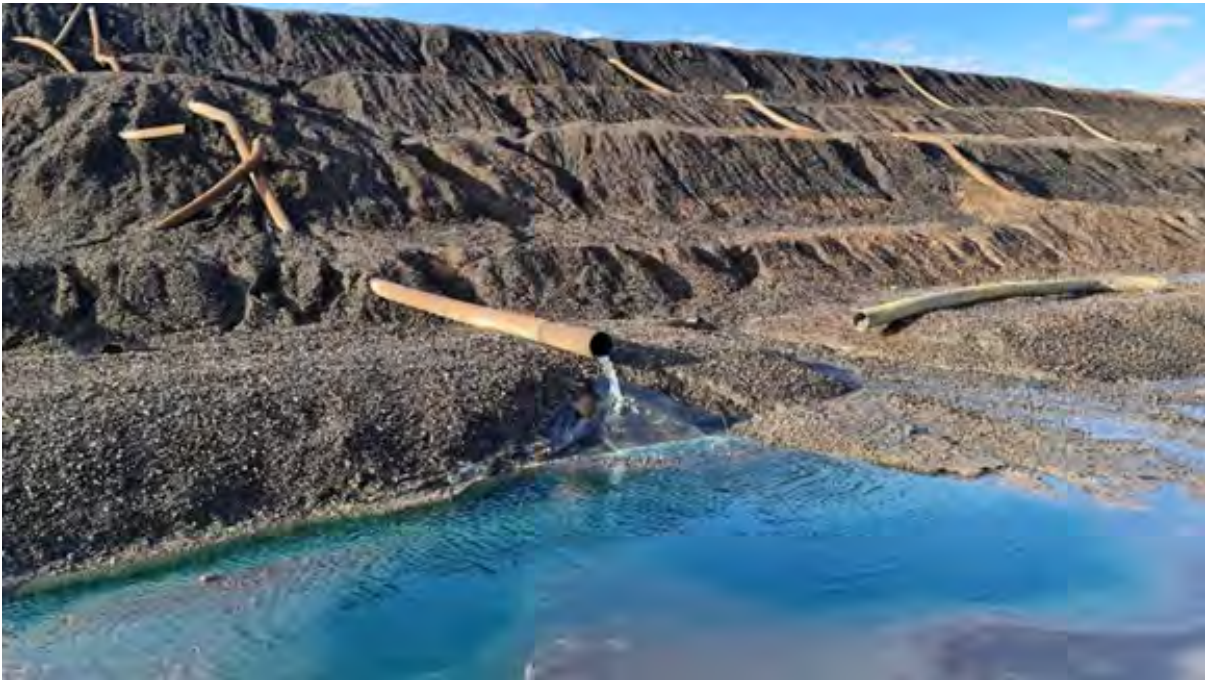
Image 7 / Copper rich solution flowing out of the heaps following recent rainfall at Nifty
