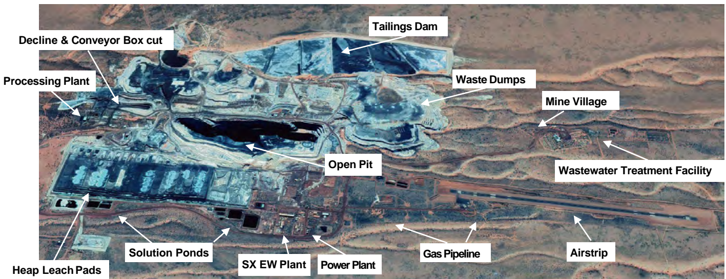
Figure 6 / Nifty Copper Mine Site Layout
