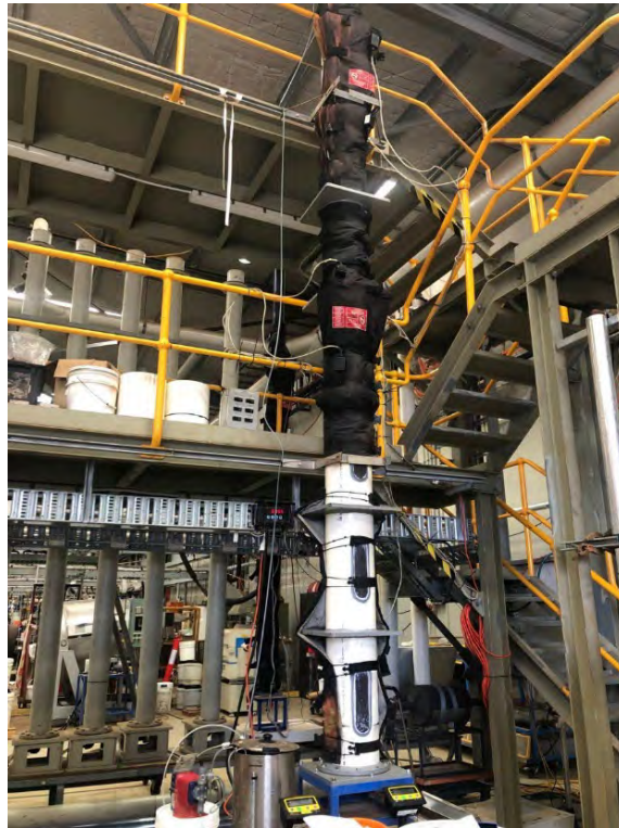
Image 11 | Nifty 6m high metallurgical test work column
