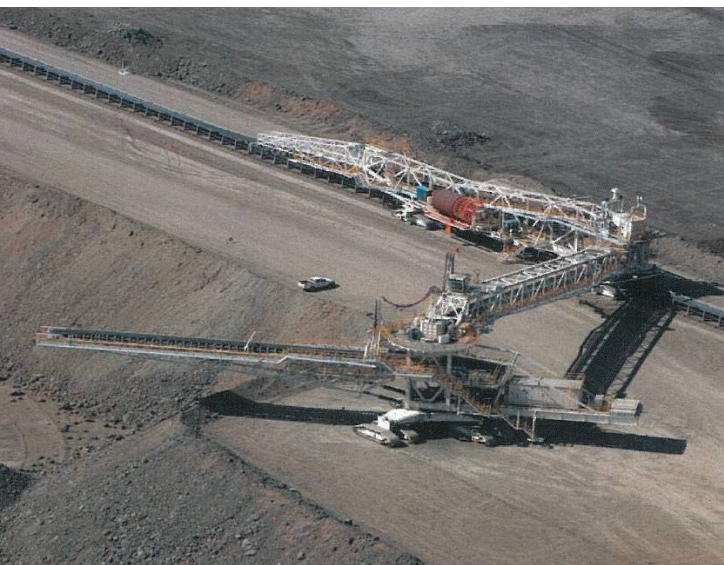
Figure 8: Dry waste stacking using spreaders. A similar process will be adopted for the Integrated Waste Landform (IWL) at the proposed mine site.
