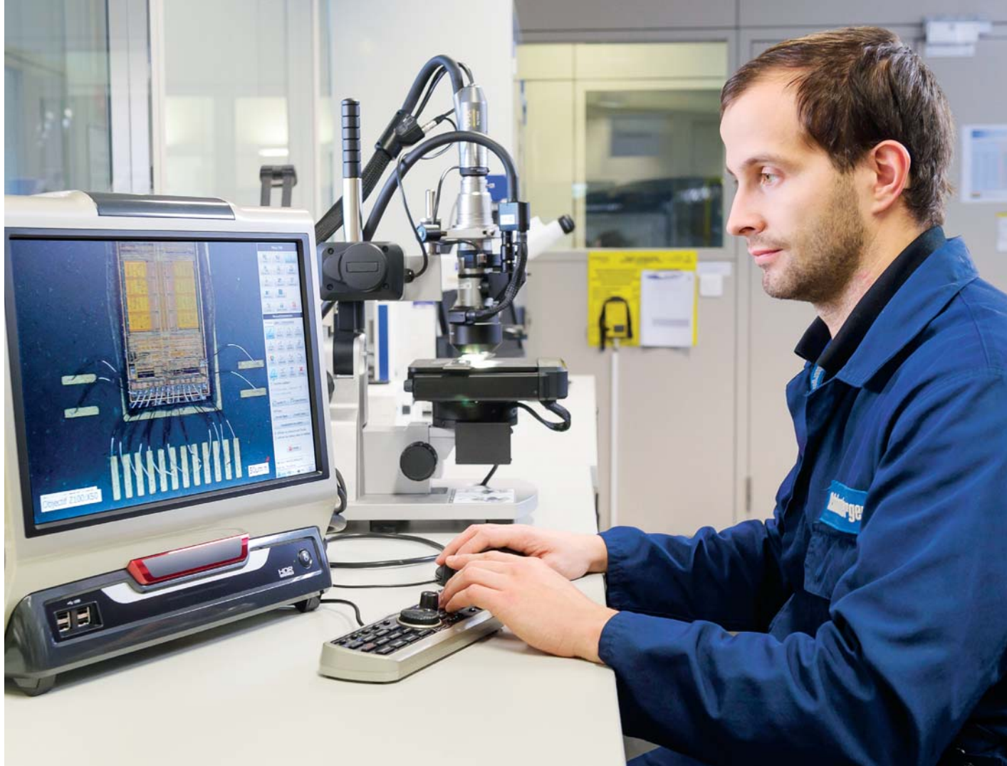
Oilfield technology is subject to environmental conditions, such as high temperatures and pressures, severe mechanical shocks, and vibration. Electrical Technology Engineer Guillaume Deville examines internal components of an electrical circuit board in Clamart, France, using a high-resolution optical microscope to identify potential weaknesses following qualification testing.
