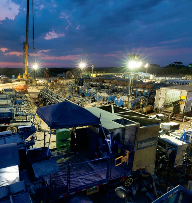
Well Services pressure pumping equipment deployed on a wellsite in South Texas in the Eagle Ford Shale play. The site is prepared for a hydraulic fracturing operation using BroadBand unconventional reservoir completion services.
