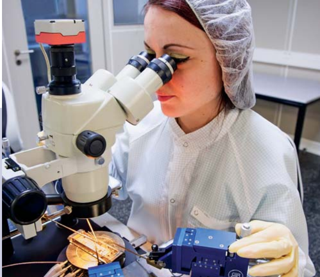
Senior Electrical Engineer Alexandra Deshayes uses a high-resolution microscope to examine an ICE sensor board to identify potential weakness following ultrahigh-temperature testing in Clamart, France.
