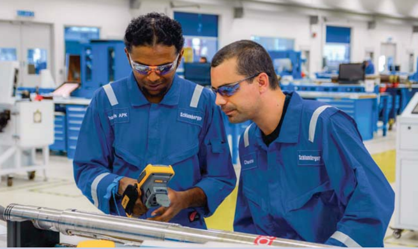
Electronic Technician Thaanis Kanason and Maintenance Expert Nicolas Laporte investigate the electronics of TeleScope* telemetry-while-drilling service by using a thermal camera in the Asia CRE in Port Klang, Malaysia. Testing for unusual thermal patterns is a proactive quality check before the tool is deployed downhole.
