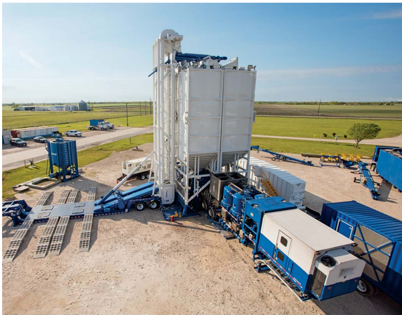
The automated stimulation delivery platform shown above incorporates a self-contained proppant delivery and storage system that streamlines OneStim materials management; improves health, safety, and environmental performance; and increases operational efficiency.
