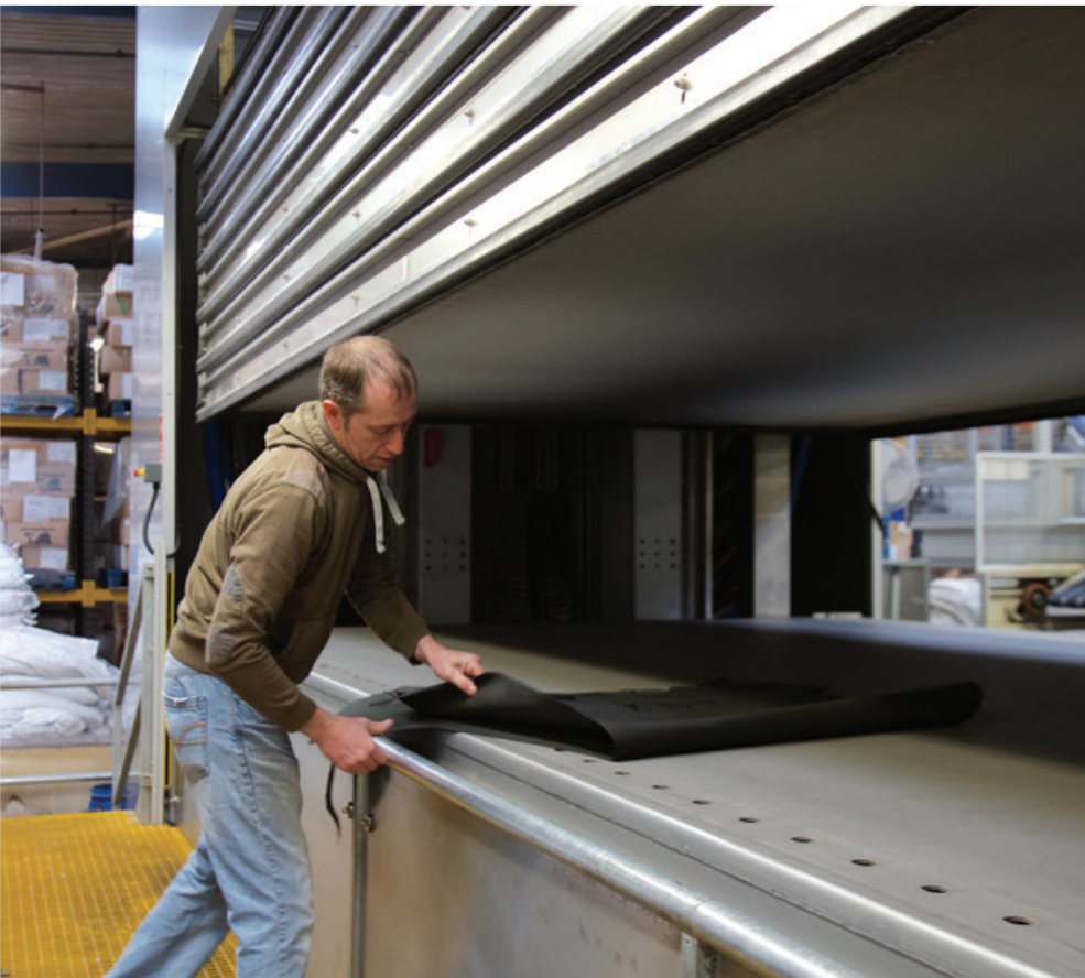
Vacuum line dryer at Yeovil
