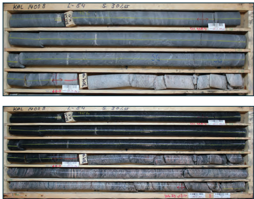
Figure 3: Dry (top) and wet (bottom) pictures taken of the logged drill core box before shipment to ALS Piteå for cutting and sample preparation for assay.
