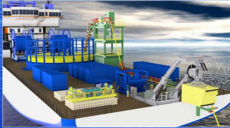
Vessel Back Deck Equipment Design (SIL)
