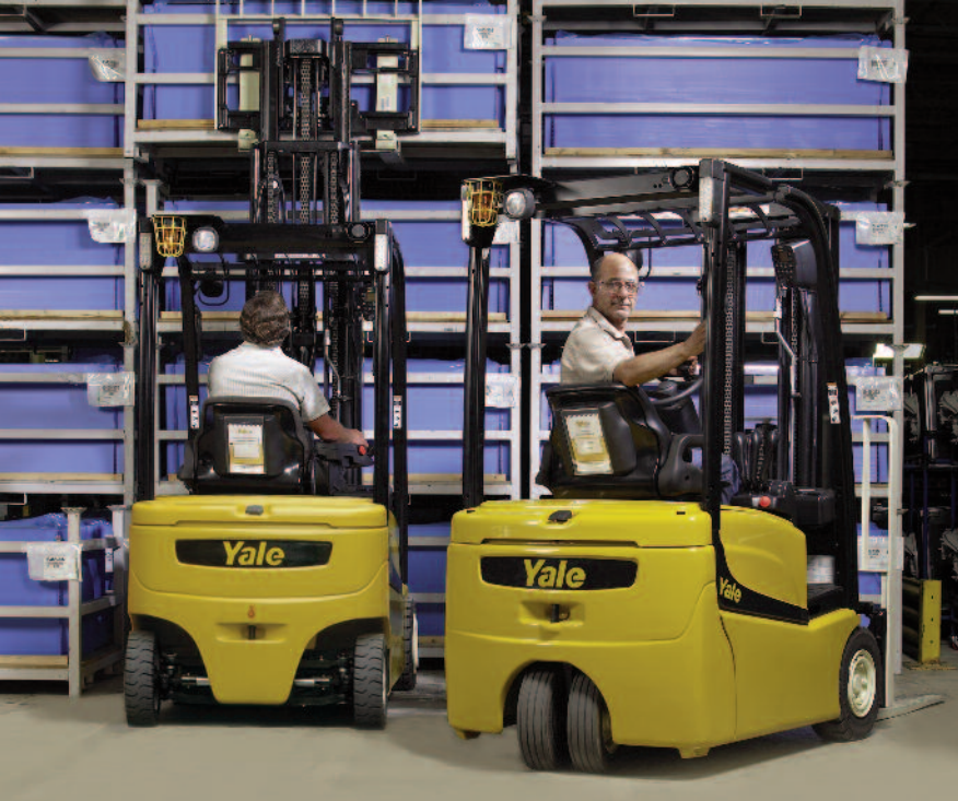
Left: Yale's new electric-riding lift truck series, the Yale® ERP-VF four-wheel (left) and ERP-VT three-wheel (right) pneumatic tire series, have lifting capacities of 3,000 to 4,000 pounds. These trucks have been designed for overall productivity at lower costs.
