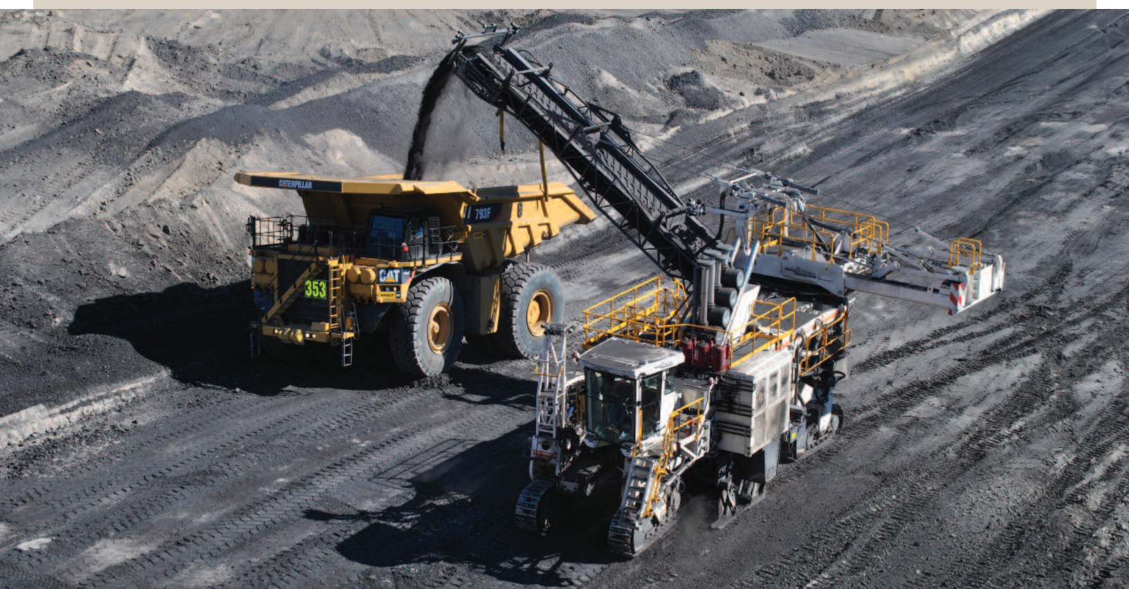
Camino Real Fuels' Eagle Pass mine in Texas began delivering coal to its customer in 2015. A Wirtgen® surface miner is used to extract coal, ensuring specific quality parameters are met.
