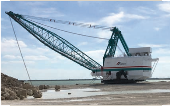
A dragline operated and maintained by NACoal's North American Mining division excavates limerock from a quarry in Florida. North American Mining expanded its Florida dragline services business in 2016 by extending an existing contract and entering into a contract with a new customer.
