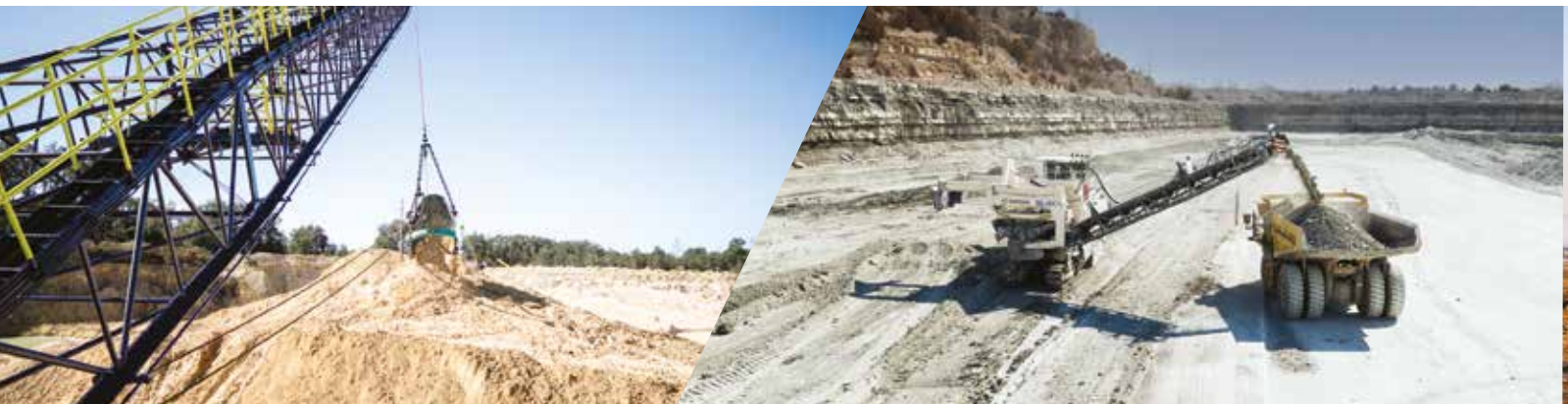
Below, a North American Mining dragline operates in Florida (left), while a surface miner works in Nebraska (right).
