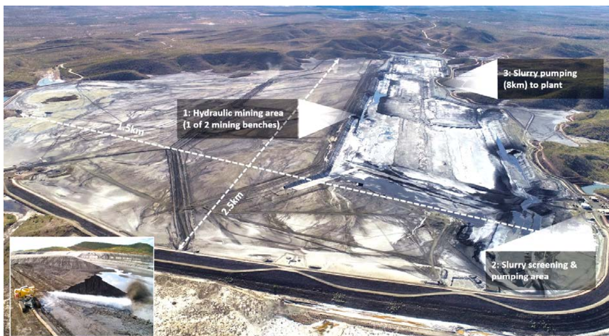
Figure 2: Overview of hydraulic mining at the Century
