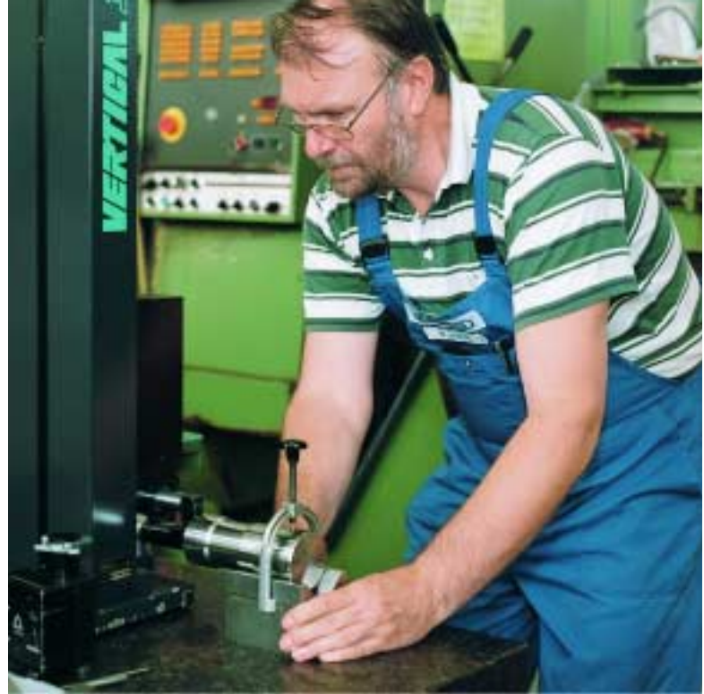
Pump Cylinder Cell Operator Wolfgang Jasyk from the Woodward Diesel Systems Center of Excellence in Aken, Germany, checks the body of a high-pressure fuel injection electro-hydraulic control valve for use on natural gas engines.
