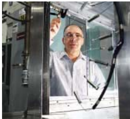
At our facility in Zeeland, Mich., Gary Bloomfield runs a flow test on a fuel manifold ring for an LV100 gas engine, which will power the U.S. Army's M2 Abrams main battle tank.
