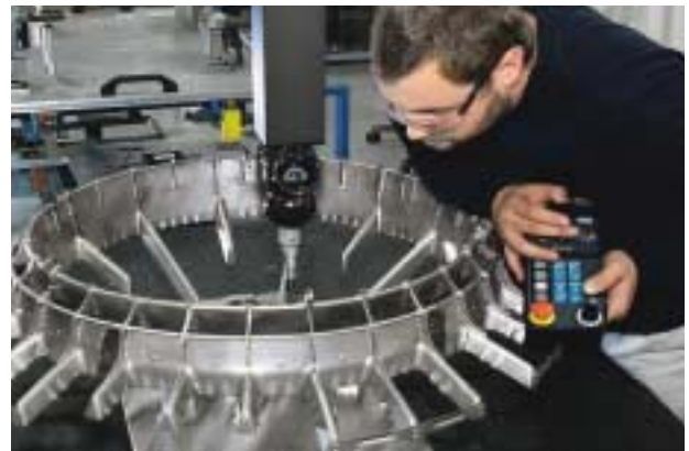
While using a coordinate measurement machine, Matt Furtaw from Zeeland, Mich., checks the dimensions of the F100 flameholder.
