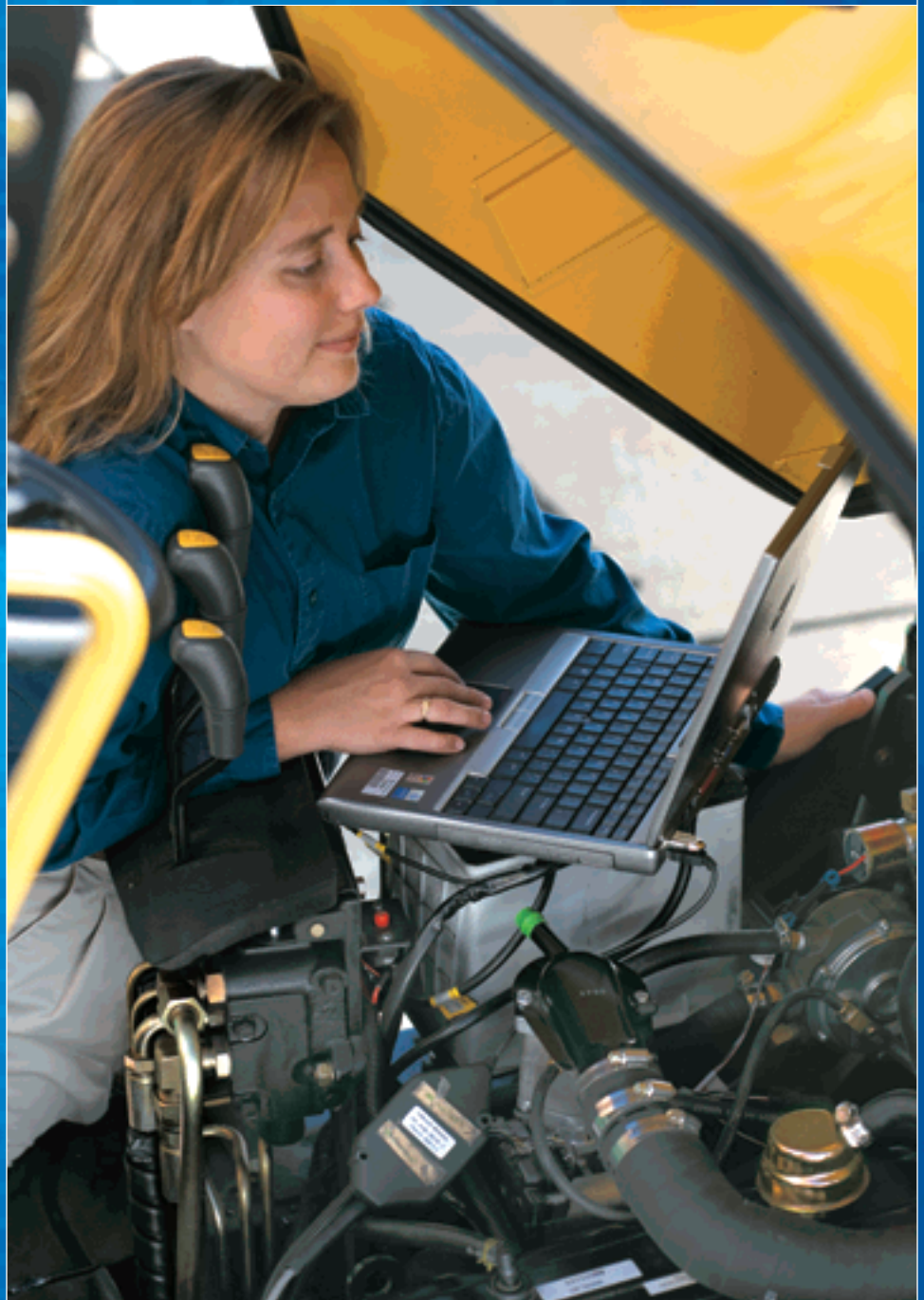
Applications Engineer Julie Fuller fine-tunes the engine emissions calibration settings on the MI-04 control system installed in a customer's prototype forklift vehicle at Woodward's engine development lab in Loveland, Colo.
