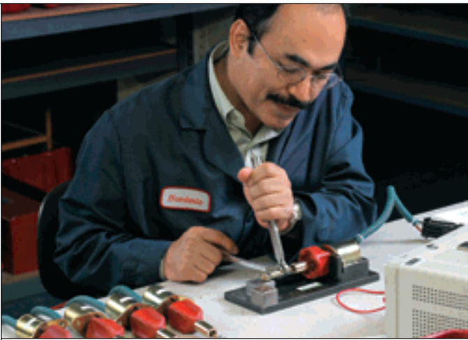
Humberto Bustamante sets the linkage adjustment on fuel control solenoids at Woodward's facility in Niles, Ill.
