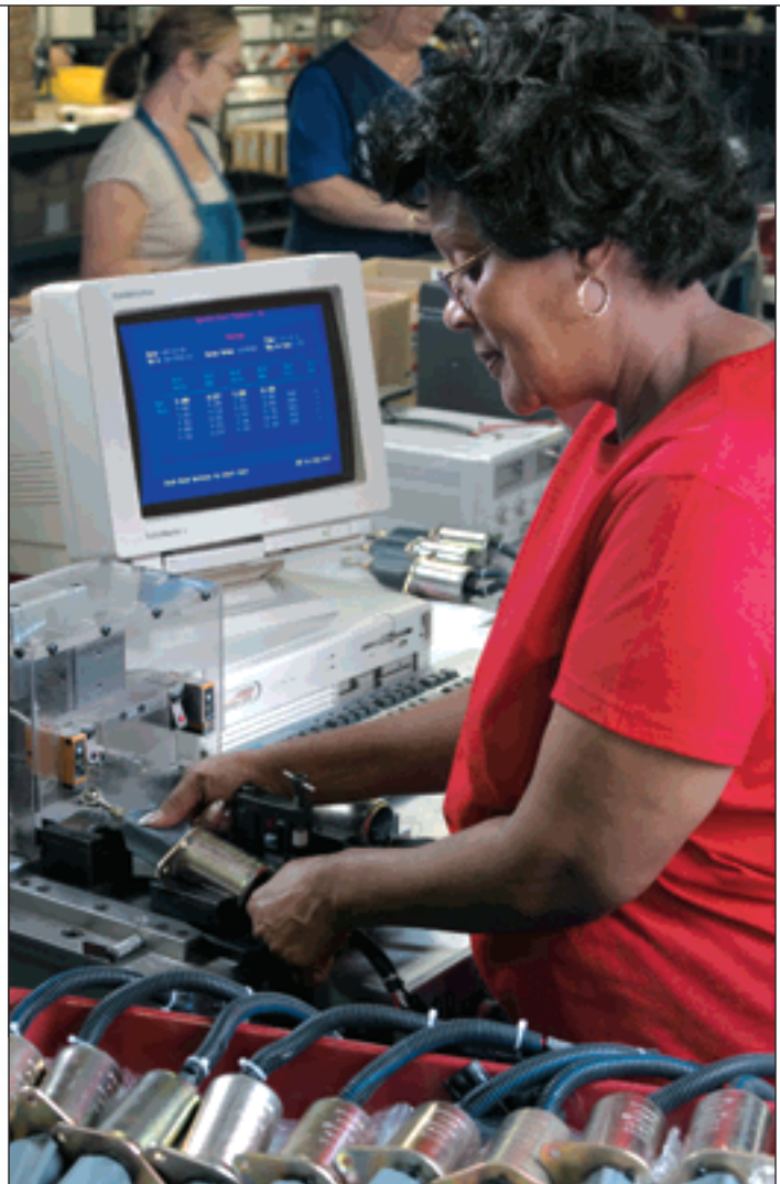
Ruby Campbell performs final testing on a fuel control solenoid at Woodward's facility in Niles, Ill. The solenoids are used in engines for off-highway agriculture, construction, utility, power generation, truck, bus, and marine applications.
