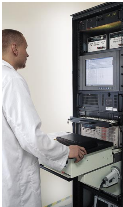
◀ Dariusz Glód, Woodward test technician, operates a test stand that checks electronic control modules (lower left) and electronic distributor modules— heavy duty (lower right). The modules are part of Woodward’s OH systems, which help reduce emissions for on-highway, heavy-duty natural gas engines.
