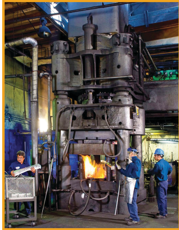
One of QAF's aluminum forging presses during a forging process
