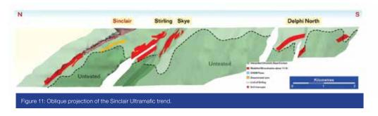
The remodelling of the ultramafic/basal contact in the near mine environment identified multiple mineralised positions, reaffirming the high prospectivity of the Sinclair Trend including the Delphi North Prospect (Figure 11).
